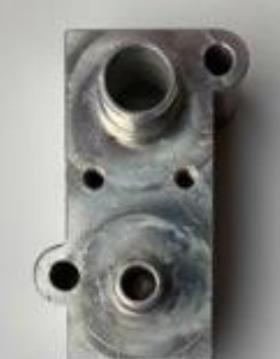
Not correctly melted ring
