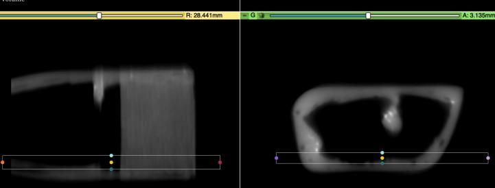
**Spectral Scan** increase recognition possibility of different materials inside propeller for better evaluation (ex. glue distribution). Photon counting detector used by RadalyX allows to recognize different materials and SW highlights
