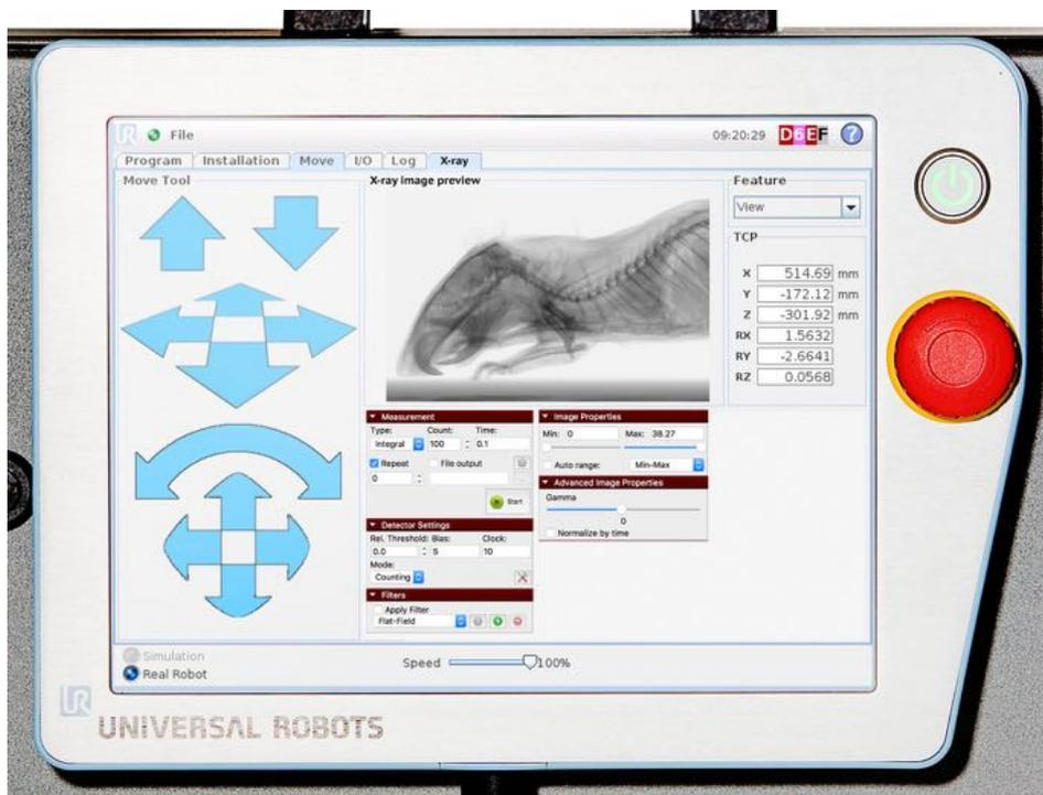
**Fig.7** A possible implementation of the detector & X-ray tube control into the PolyScope software operated by the portable touch screen of the Universal Robots controller. The robot movement control buttons remain accessible for online change of the X-ray view direction.
