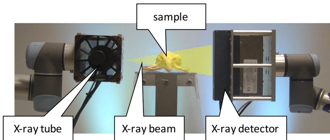
**Fig.2** Detail of the X-ray imaging setup: X-rays generated in the X-ray tube are passing through the sample and are detected by the imaging detector. The intensity of X-rays is changed by the sample to different levels revealing the internal sample structure.
