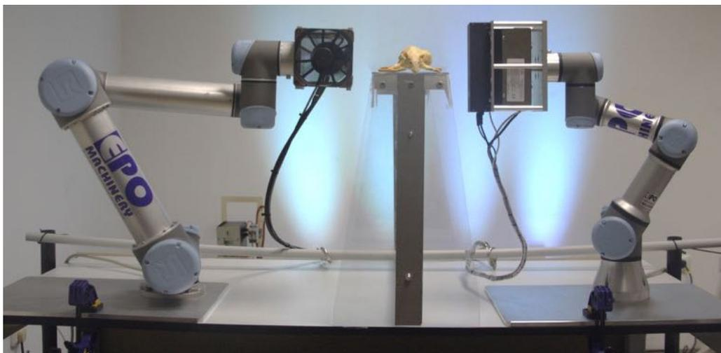
**Fig.1** A pair of robotic arms holding X-ray tube (left robot) and X-ray imaging detector (right robot). The imaging test was performed in this case for small animal imaging for pre-clinical research of new drugs and cancer treatment techniques.
