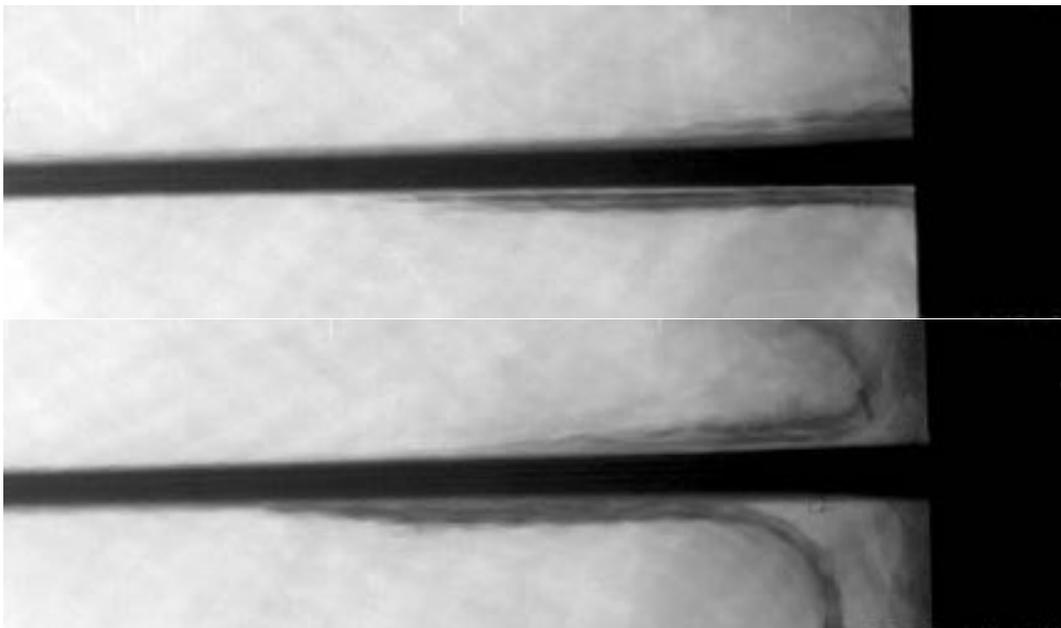
**Fig.12** A steel pin inserted into the composite viewed from two angles. It clearly reveals differences of pin fixation into the aileron in each direction.
