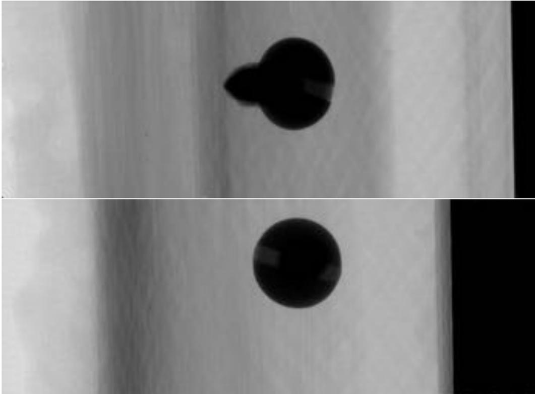
**Fig.11** Screw inserted into the composite easily viewed from two angles.
