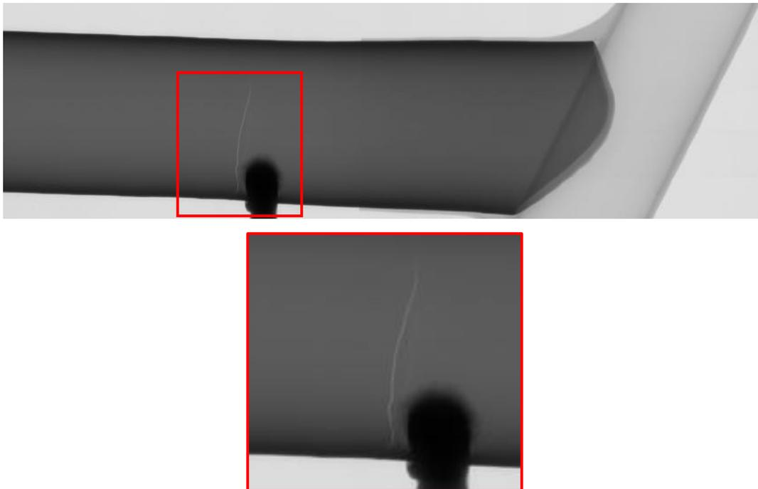
**Fig.6** Final X-ray image of the scanned frame and detail of the identified crack in the titanium pipe.
