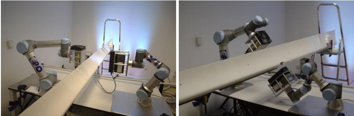
**Fig.9** Flexibility of the robotic system is demonstrated on inspection of a glider aileron: besides 2D scanning (left image) it is possible to inspect critical parts of the aileron, such as joints, under arbitrary angles (right) revealing locations of defects otherwise hidden in the 2D scan.
