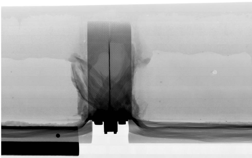
**Fig.10** Final X-ray scan of the selected area of the glider aileron. The darkest areas are metallic parts inserted into the composite aileron. Inspection of quality of their fixation into the composite is therefore difficult without angular views.
