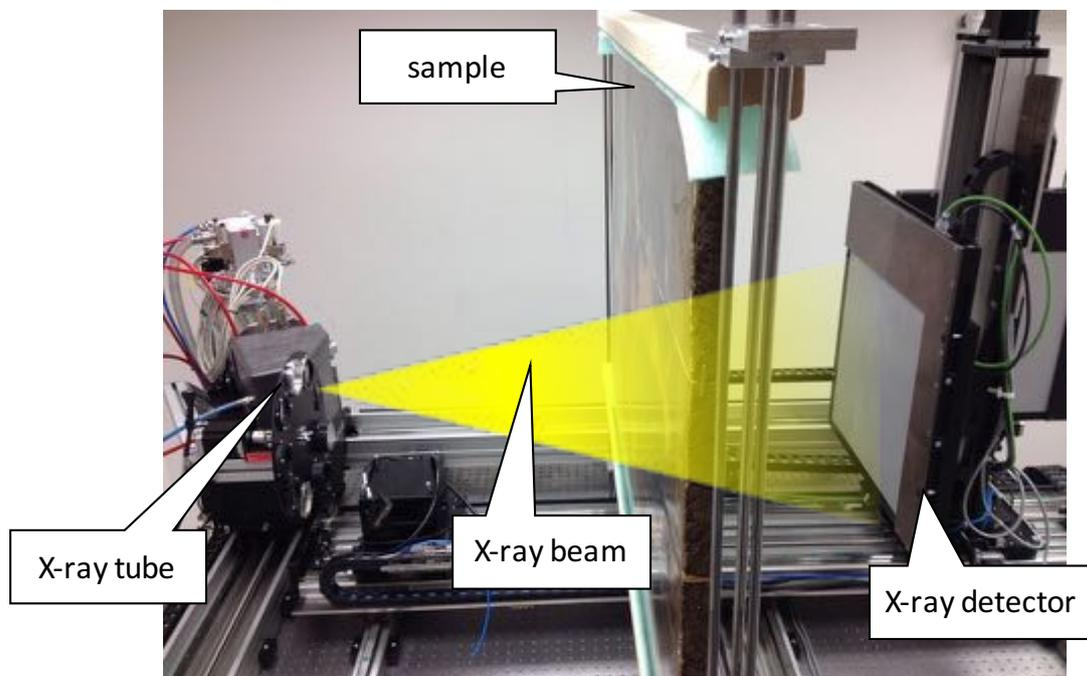
Fig.4 A typical X-ray imaging setup where the X-ray tube and detector can move only linearly => very reduced range of imaging angles limiting the possibility to visualize some defects or internal sample structures.
