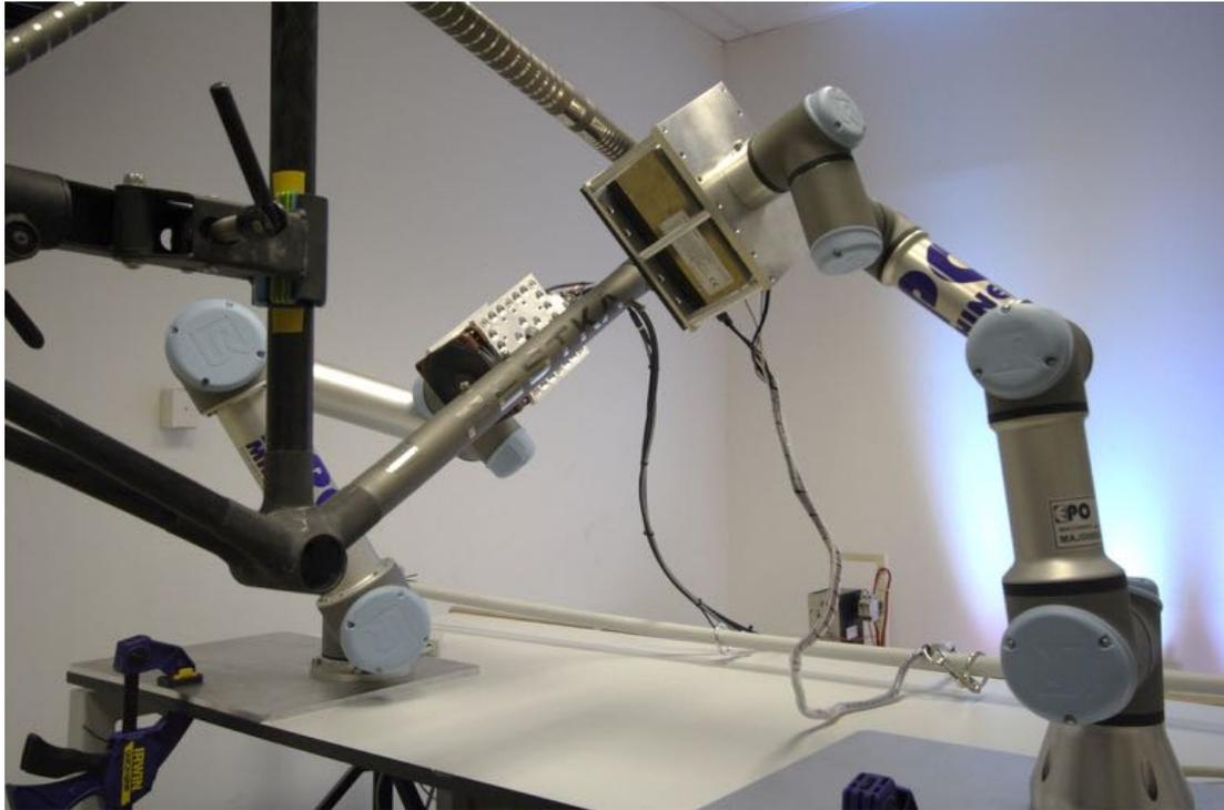
**Fig.5** Robots inspecting a high-performance bike frame for defects. The bike frame is a typical sample which takes advantage of robotic system – it is necessary to inspect only relatively small areas that are parts of a large structure.
